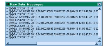
by the individual data fields, decomposed into their true contents. Some messages may only be partially decoded, the missing fields designated with ellipsis (. . .). Messages which are not decoded at all, such as those marked with a ?, have only the message identification characters shown (the first four characters in the case of a Motorola receiver).
