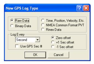
The **Raw Data Log** will contain the messages from the GPS receiver preceded by an input or output arrow. Binary data messages will be interpreted.
