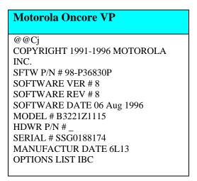
The Motorola message is only received once as part of initializing the receiver. This happens when SynTac is started and again every time the OK button is clicked in the serial port settings dialog box. This information is derived from a binary message even if the receiver is set to NMEA mode because there is no equivalent NMEA message for the Motorola GPS receiver.
