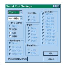
and should accurately reflect the available COM ports on your computer. This includes both normal and high performance ports such as those that are part of RISC and ASIC processor boards. Ports are listed here even if they are in use by another program. If you choose a port that is already in use an error message will appear.
