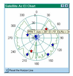
will appear as lines radiating from the center to each active satellite. Over time the horizon trace will fill in as satellites move through their orbits. It takes at least twelve hours to complete a horizon trace as shown above. Note that in this trace several large trees block the satellites between 150 and 190 degrees azimuth. No satellites are seen at low altitudes to the north because of their orbit inclination relative to the latitude of this station (about 39 degrees North).
