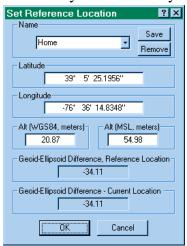
reference locations to be preprogrammed for later recall. Selecting a name from the drop-down list will cause all the fields to be filled with the information associated with that name. To update a database entry, change the data and press the Save button. To create a new entry, enter a new name and press Save. To remove an entry, choose the entry from the drop-down list and press the Remove button.
